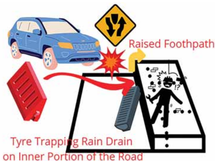
Image 1: Suggested methods to prevent vehicle tyre getting over footpaths in urban areas.
